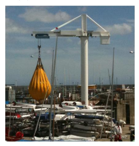
The water weight above is of 20 tonne capacity and was filled to 16.75 tonne for that particular test.
